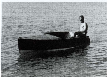
The COMET when owned by the Welch family of Kerikeri. Note the batten-seam topsides and the high chine and hollow entry forward.
