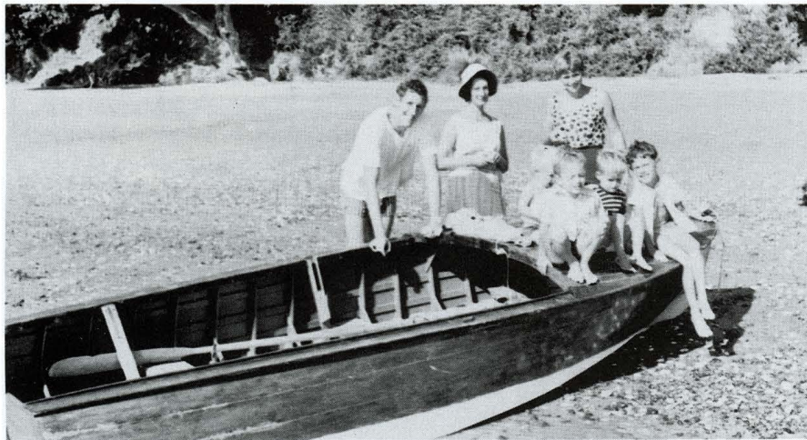
The COMET when owned by the Welch family of Kerikeri. Note the batten-seam topsides and the high chine and hollow entry forward.
